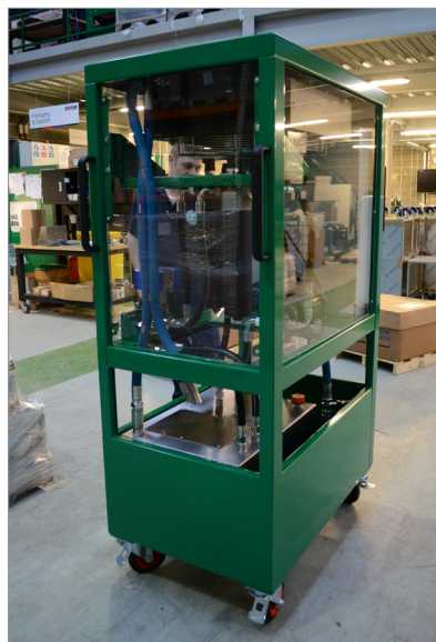
Hydraulic Motor Testing Station
